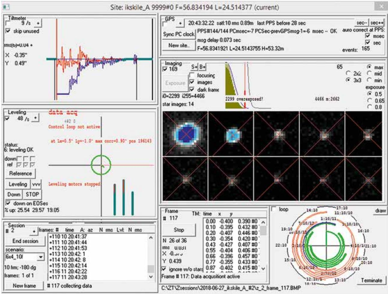
Fig. 3. Session control panel. Clockwise from top left – tiltmeter controls, GPS and timing controls, CCD and star image controls, session scenario, frame data acquisition, session data acquisition, levelling and rotation controls
