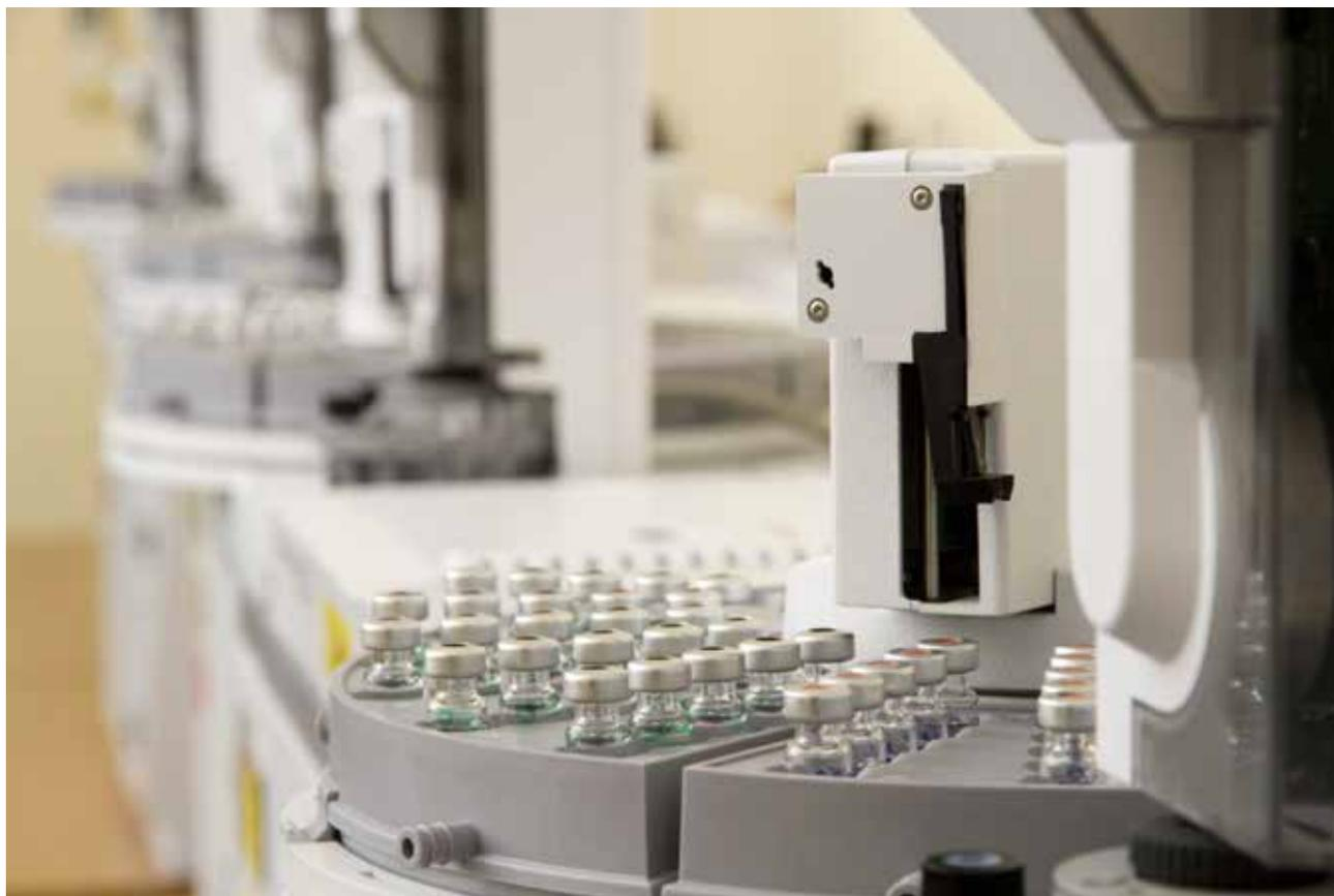
Fig. 6. Sample preparation for chemical analysis using liquid chromatography-mass spectrometry method
