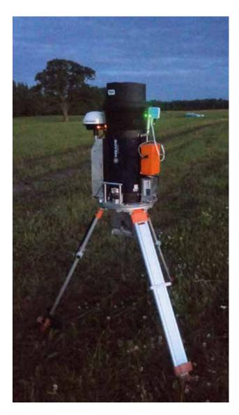
Fig. 1. Digital zenith cameras for observations at night
